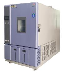
The programmable constant temperature and humidity test chamber is a versatile, essential device. It precisely simulates high/low temperature and alternating humid environments products, materials, and packaging may face during transportation, storage, and use. By exposing them to these conditions, it effectively assesses their resistance to heat, cold, and humid - heat, helping manufacturers and researchers spot weaknesses.
